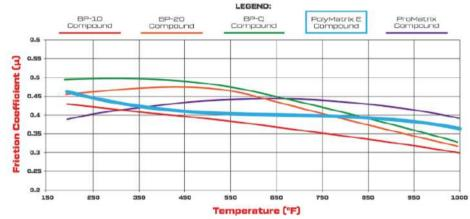
PolyMatrix E Friction Coefficient and Temperature Values
